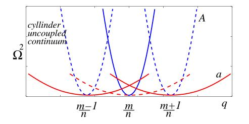
Alfvén/acoustic coupling in toroidal equilibrium (schematic)
