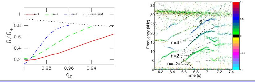
NOVA predicts  $f_{BAAE} = 24.8kHz$  against observed 14kHz, all *n*'s exist ( $q_0 = 1$ ). Possible way to resolve this is to assume local negative shear with  $q_{min} = 3/2$ : 1) frequency  $\sim q^{-1}$ , goes down to  $\sim 16kHz$ , 2) only even m's are expected:  $m = nq_{min}$  is integer.
