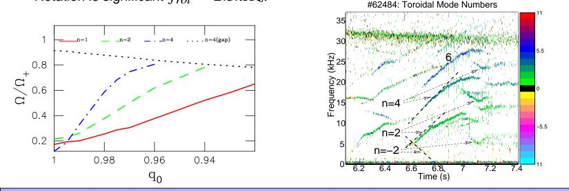
NOVA predicts  $f_{BAAE} = 24.8kHz$  against observed 14kHz, all *n*'s exist ( $q_0 = 1$ ). Possible way to resolve this is to assume local negative shear with  $q_{min} = 3/2$ : 1) frequency  $\sim q^{-1}$ , goes down to  $\sim 16kHz$ , 2) only even m's are expected:  $m = nq_{min}$  is integer.
