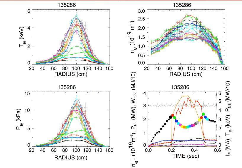
P<sub>RF</sub> programmed up to 3.7 MW without arcs after conditioning of previous day
