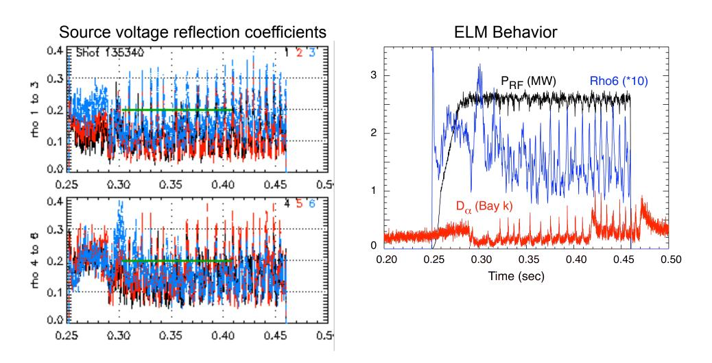
Coupling through ELMs possible if trip value of rho can be set to a high value (0.7 in this case)
