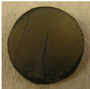
ATJ147a 2000 nm Li deposited, 1.5 hr D irradiation
