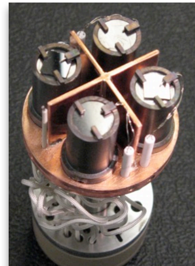
Fig. 1 Sample probe with ATJ graphite, Si and Pd samples
