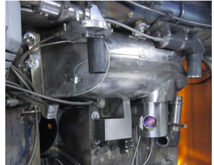
MSE periscope covered with radiative heat shield
