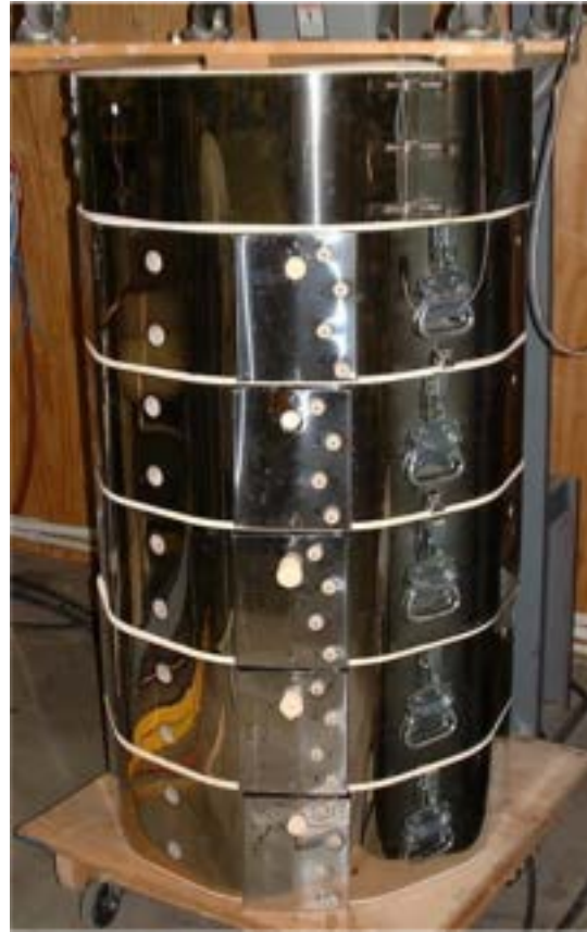
Zoned stack furnace (extendable to 4 m)
