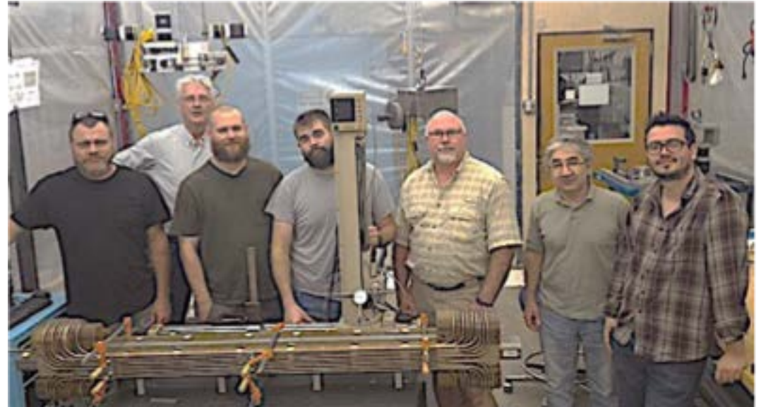
Completed 24-turn winding for 1.2 m dipole.
