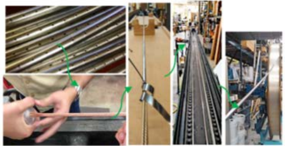
Fabrication of 1- and 10-m CIC segments at ATC.
