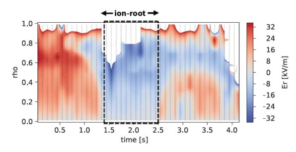
First measurements of the ion-root in W7-X plasmas made possible by XICS diagnostic.
