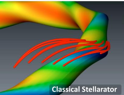
Shown is the orbit of a 50 keV ion in a optimized stellarator of similar size and design as W7-X. This energy scales to an α-particle in a reactor scale device.
