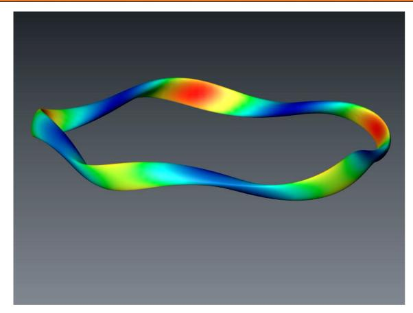
Shown is the orbit of a 50 keV ion in a optimized stellarator of similar size and design as W7-X.
