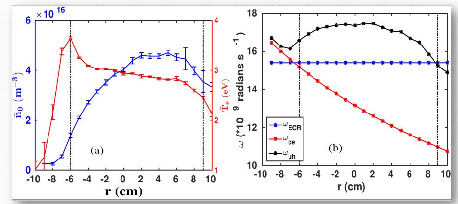
• The profile of (a) mean density  $(\bar{n}_0)$  and mean electron temperature  $(\bar{T}_e)$  and (b) upper hybrid resonance,  $\omega_{UH}^2(r) = \omega_{ce}^2(r) + \omega_{pe}^2(r)$ .
