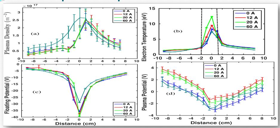
Radial profiles of (a)density, (b)electron temperature, (c) floating potential and (d) plasma potential are shown here.
