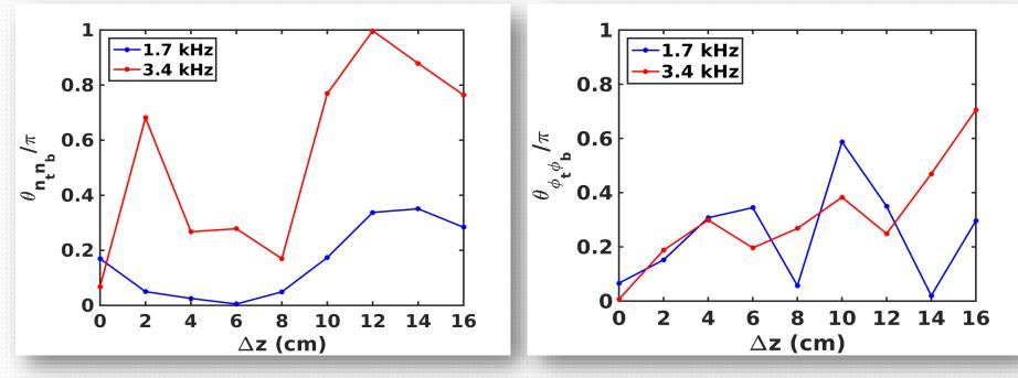
• The phase for density fluctuation for 3.4 kHz is  $0.8\pi$  or more beyond  $\Delta Z = 10cm$ .
