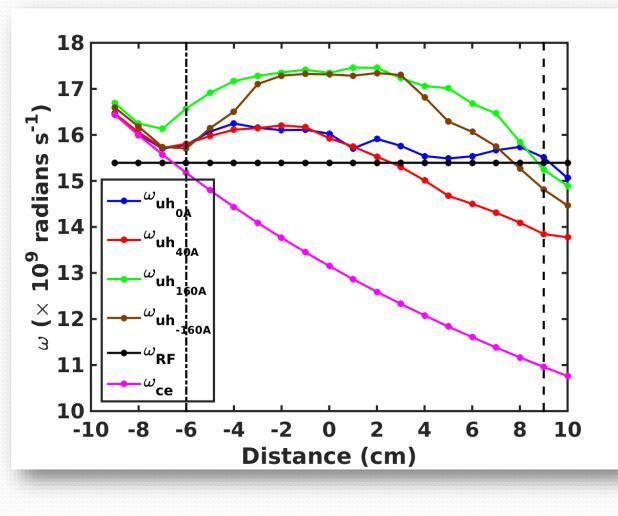
• Radial profile of the upper hybrid resonance for different VF current.
