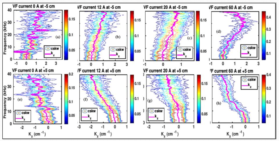
Contour plots of conditional spectrum  $S(k,\omega)$  with embedded line showing vertical wavenumber ( $k_z \text{ or } k_\theta$ ) estimated four VF currents at -5 cm and +5 cm.
