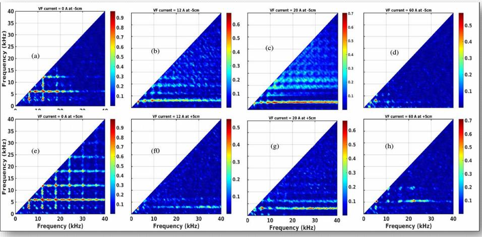
Bispectrum of  $I_{sat}$  fluctuation for single shot for VF current of oA, 12A, 20A, and 60A at -5 cm and +5 cm.  $b^2 > 0.9$  for oA and reduces further for higher currents. These plots are zoomed in up to 40 kHz.
