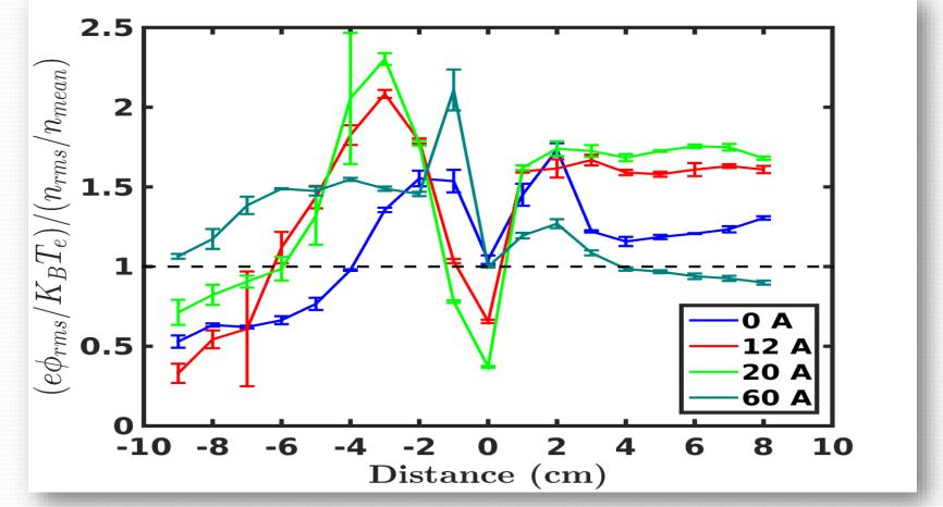
Radial profile of ratio of relative potential fluctuations to relative density fluctuations.
