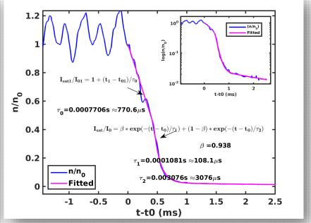
Density fall for ECR source for 160 A or short connection length case. Density shows linear fall followed by exponential fall, after the source is turned off.
