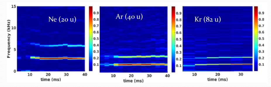
• In order to confirm the acoustic-like nature  $(f_{TAM} \propto 1/\sqrt{M_i})$  of the observed mode, the ion mass has varied.
