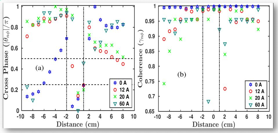
• Cross phase normalized to of density and potential fluctuations and Coherence between density and potential for four values of VF current of 0 A, 12 A, 20 A and 60 A.
