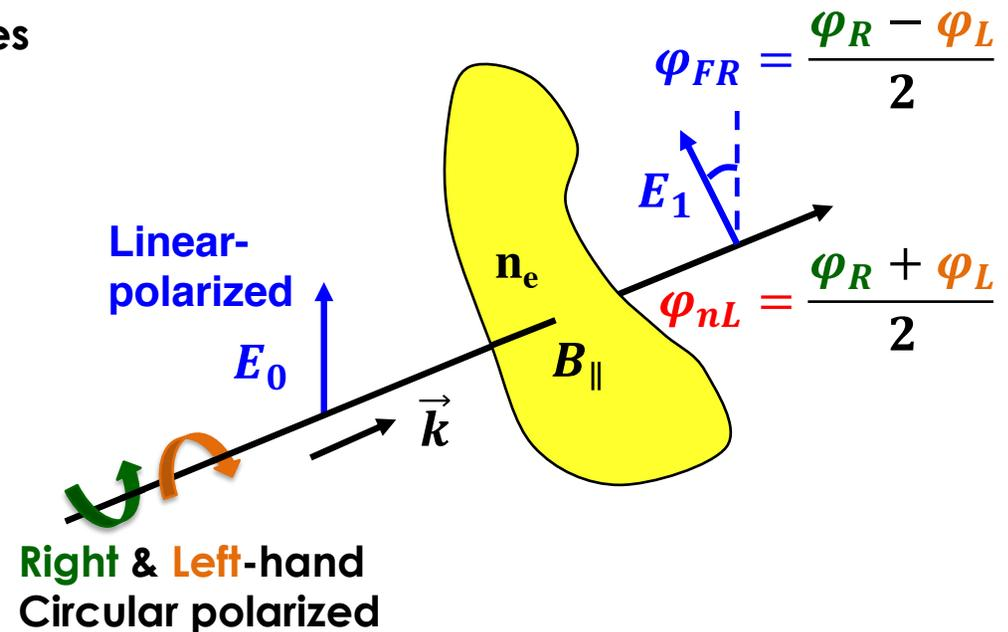
Simultaneous Polarimetry-Interferometry Measurement along the same chord
