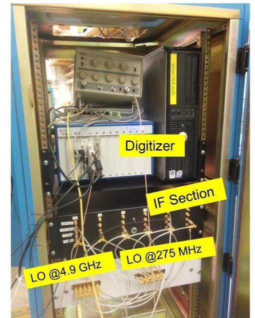
4.6 GHz power detection system at MIT
