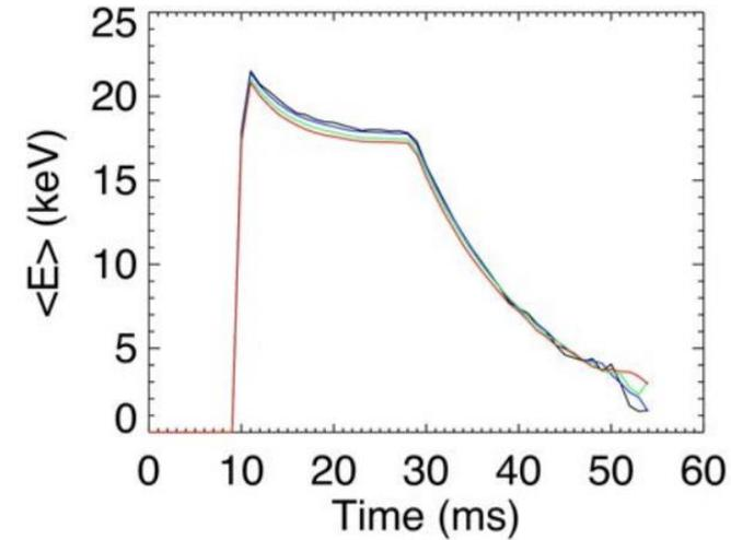
Fig. 5.13: TRANSP average fast-ion energy vs time at four radii from  $r = 0-0.2$  m shows near constancy with radius.
