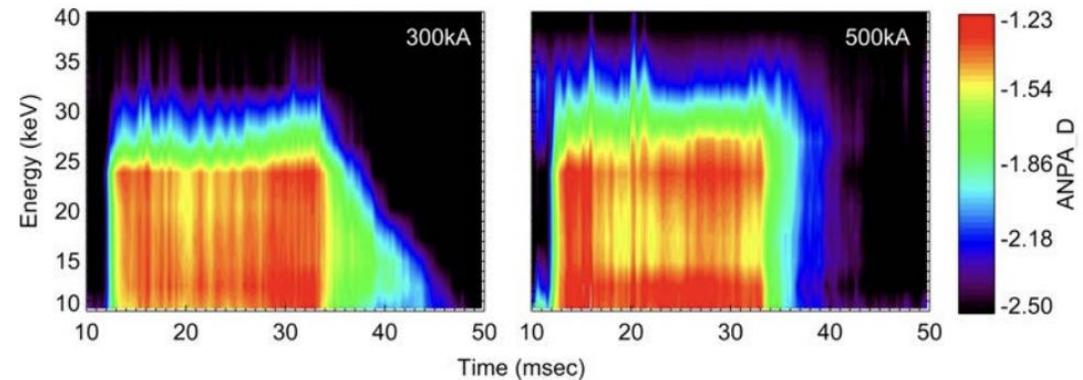
Fig. 5.14: ANPA spectrogram for 300 and 500 kA datasets. Injection near 25 keV connects through a broad profile to the lower energy channels.
