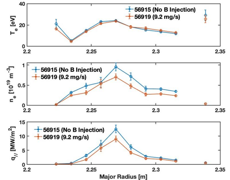
Divertor Langmuir Probe  $T_e(t)$  and  $n_e(t)$  at  $R=2.28$  m
