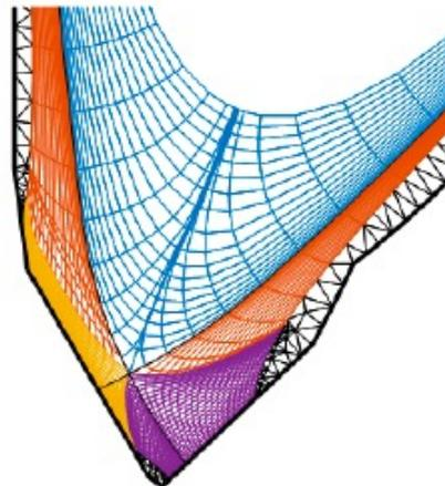
**Balanced divertor with baffling and simplified targets**
