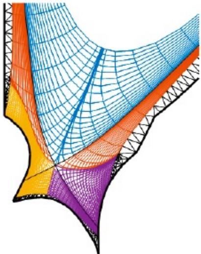
**“ITER-like” baffled vertical target divertor**
