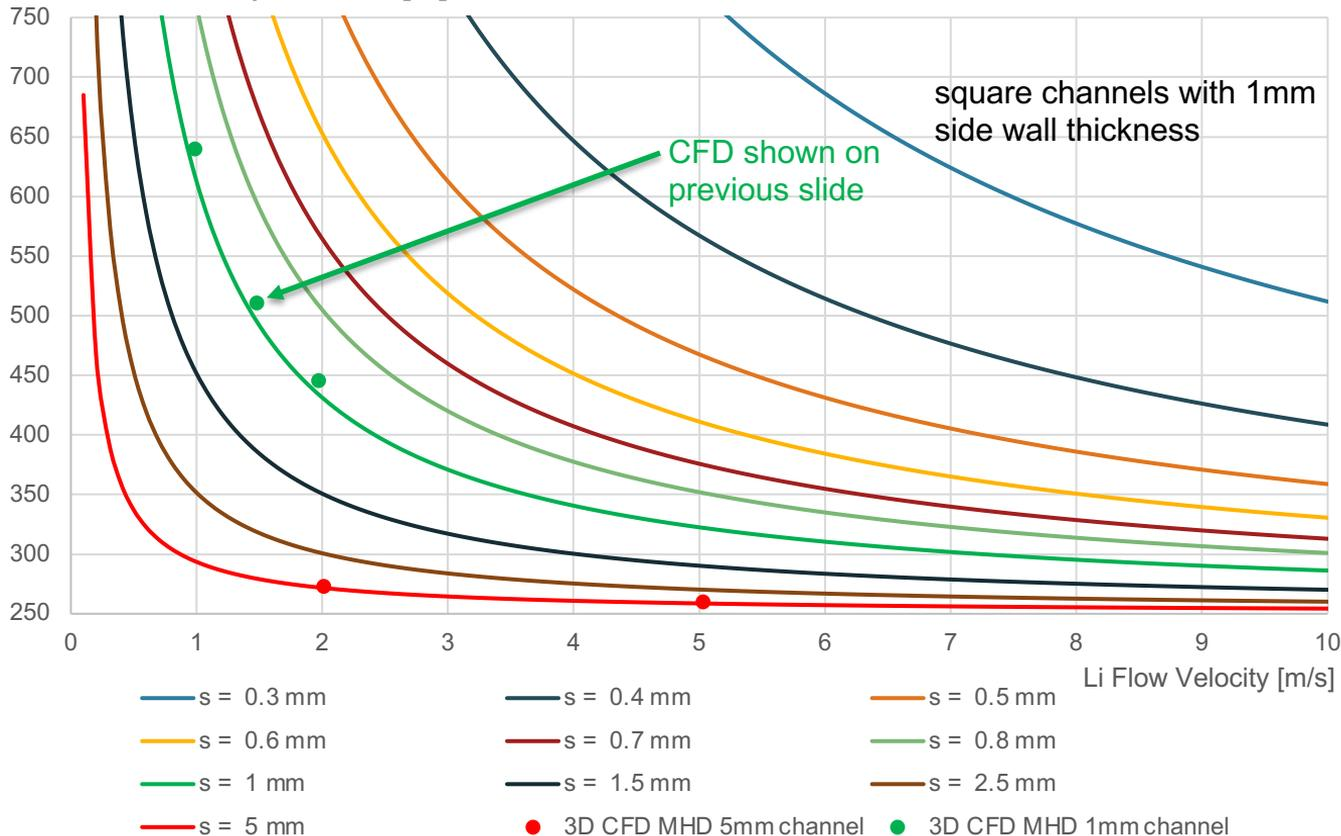
~500C temperature level is currently targeted by Vapor Box divertor System
