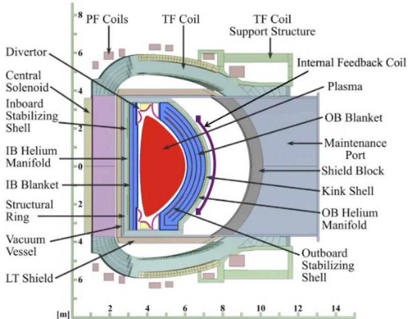
The cross-section of the FNSF, identifying the various components in and near the fusion core.
