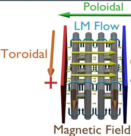
Toroidal divertorlet concept being tested
