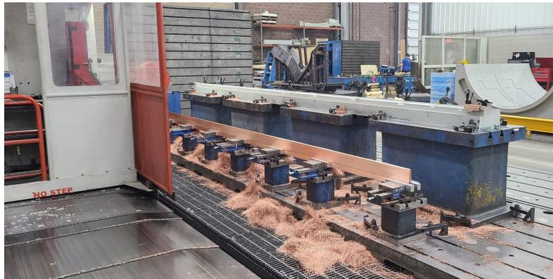
Pre-weld machining prototype @ Visioneering
