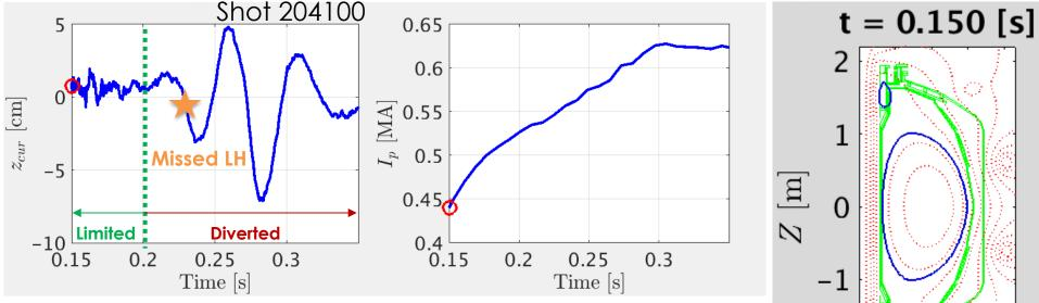
**Problem** =  $z_{cur}$  oscillation + shape dithering to/from USN/LSN prevented access to H-mode (low  $I_i$ , high performance)
