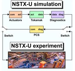
GSEvolve [4,5] plasma-response model within Tokamak is based on Grad-Shafranov equation. Actuators (H&CD, Power supply) + Diagnostics models, plus PCS
