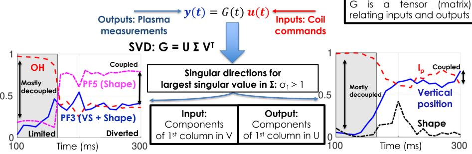
NSTX-U PCS uses "decoupled" loops, but they are not decoupled when diverted
