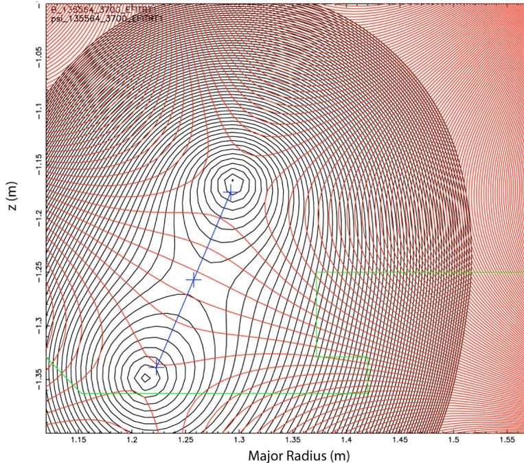
Fig. 1. Result of tracking algorithm as applied to actual data. Plotted are  $|B_{pol}|$  contours (black), flux contours (red) and the snowflake center and X-points (blue crosses). The green line corresponds to the location of the floor and shelf of the lower divertor.
