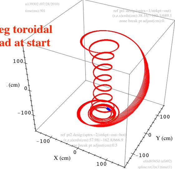
By virtue of symmetry of underlying equilibrium, angular distance between two current filaments (field lines) within a toroidal sheet is invariant: a toroidal profile imposed at divertor is faithfully replicated elsewhere including mid-plane – good for ELM triggering, but slight problem: *there is no such thing as sheet current in real life – current must have radial spread.*
