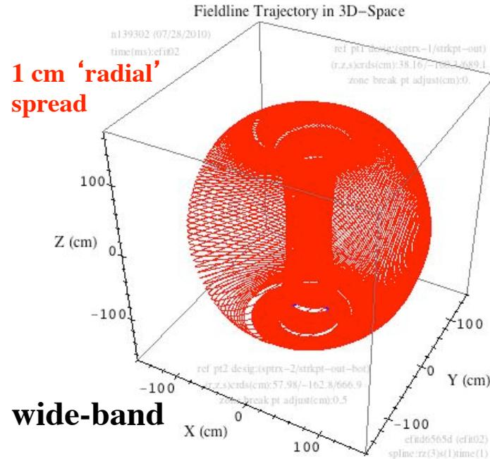
Field lines in a "high shear" region of strong differential revolution arrive in mid-plane with very different toroidal phase, and current along these field lines tend to generate largely axisymmetric field due to "phase-mixing" effect (APS '00 and NF '04). *Not good for ELM triggering, but wonderful for preserving precious axisymmetry.*
