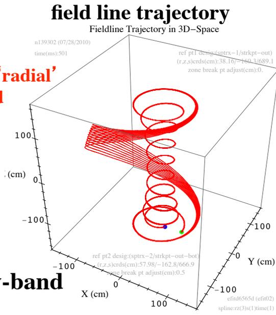
Because of singularity at a secondary separatrix, a high “shear region” next to the primary separatrix gives way to a “zero-shear point” farther away (~ 10 cm) from strike point, whereby a narrow-band toroidal spread is recovered in spite of a radial spread in starting points.
