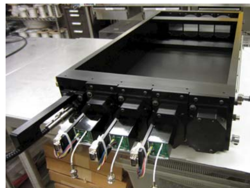
Existing prototype hardware used for imaging the x-point through coherent fibers
