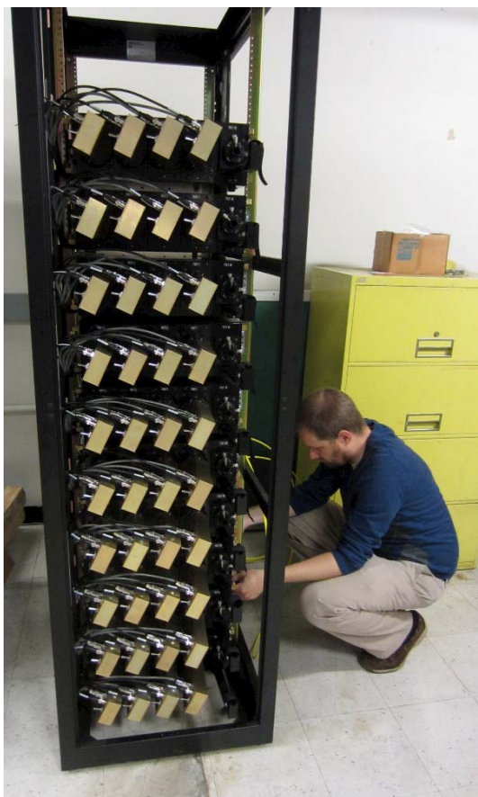
10 polychromator system for Multi-spectral MSE
