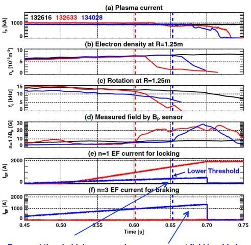
Resonant threshold decreases when non-resonant field is added
