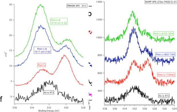
XPS scans of C-1s and O-1s photoelectron regions before and after MAPP sample exposure to an argon glow in LTX, showing the appearance of chemical shifts following the glow. **M. Lucia et al Rev. Sci. Instrum. 85, 11D835 (2014)**
