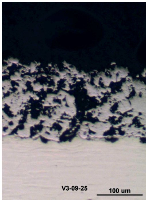
LLD surface cross section: plasma sprayed porous Mo
