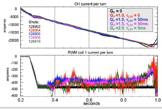
n=3 EFC + n=1 feedback important at lower current (< 900kA) for extending pulse lengths
