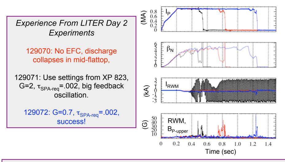
The parameters of 129072 were "locked-in" as the standard pre-programmed n=3 + n=1 DEFC.
