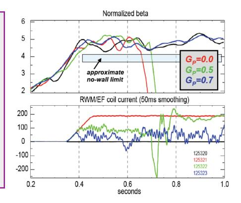
Final "Optimal" Configuration Use identification of the mode form B<sub>P</sub> sensors Use a feedback phase of ???° Use a feedback gain of 0.7
