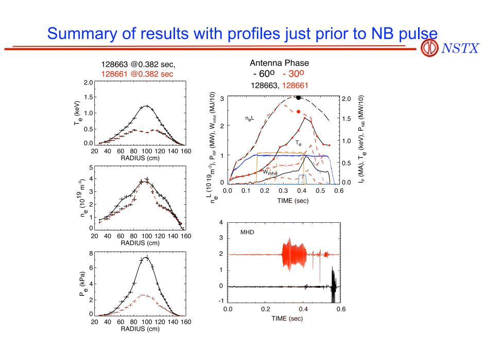
• For the large difference in heating between -60° and -30°, we might expect that the edge density during the instability should be large relative to the onset density
