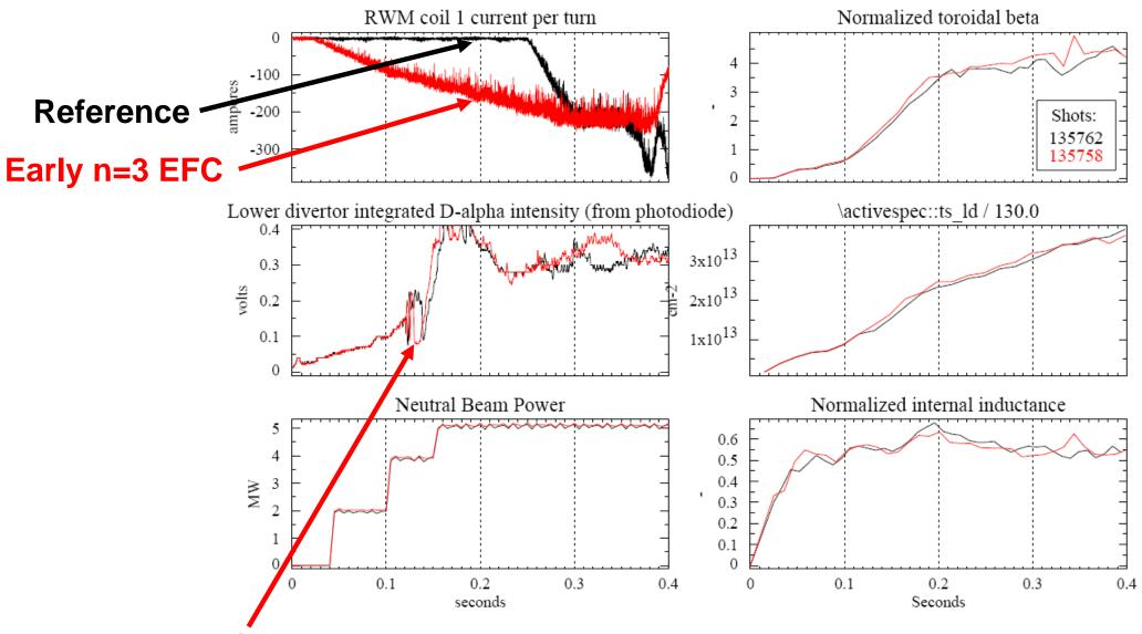
Early n=3 EFC induces earlier H-mode transition – reduced flow damping?
