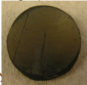
ATJ147a 2000 nm Li deposited, 1.5 hr D irradiation
