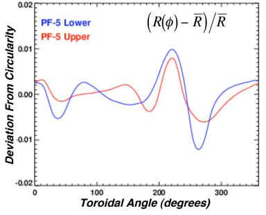
• PF-5 Coils are out of round, with a significant n=3 component.
