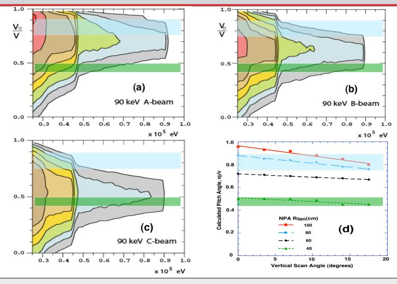
• For 'standard' settings of the NPA,  $R_{tan} \sim 70$  - 80 cm,  $v_{ll}/v \sim 0.80 \pm 0.05$  (blue bar).
