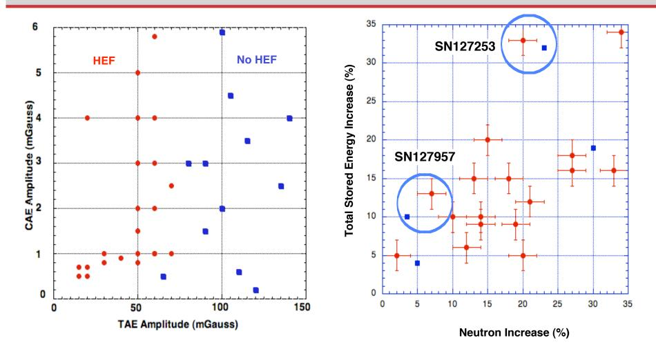
• The experimental neutron rate and total stored energy increase during the HEF (right plot). Similar increases are observed in some TRANSP analyses (blue squares).
