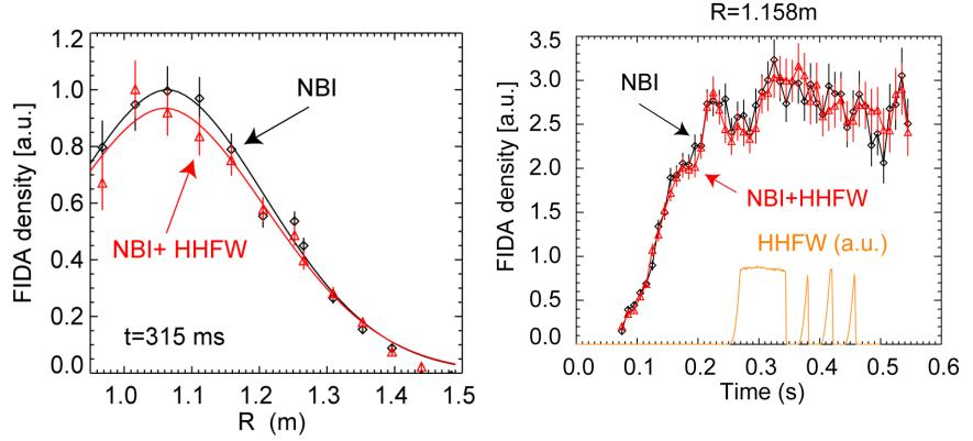
FIDA density profiles at t=0.315 s for, red, plasma with NBI+HHFW heating and, black, reference NBI-only plasma  Evolution at R=1.158m of FIDA density for, red, plasma with NBI+HHFW and, black, reference NBI-only plasma
