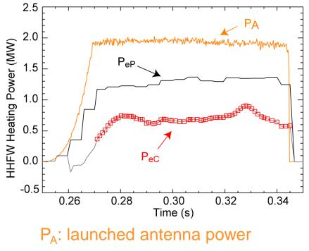
P<sub>eP</sub>: TORIC calculation of power to electrons assuming 100% capture With LCFS
