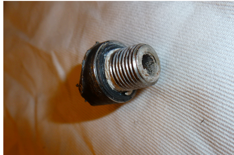
Water Fitting: Melted on one side, just “used” on the other.
