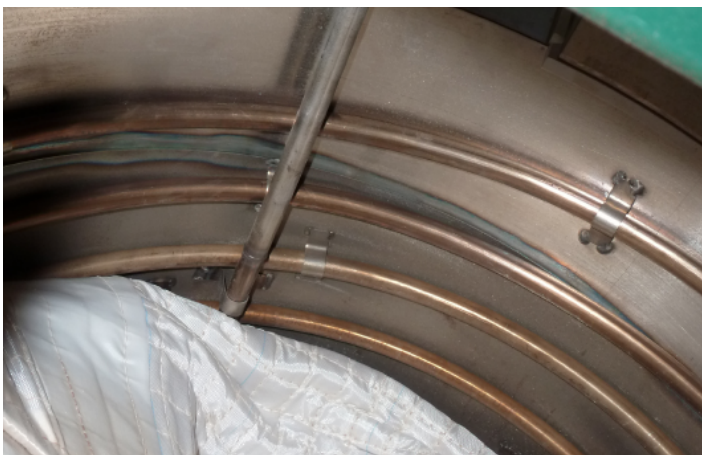
Divertor CS SS cooling tubes in NSTX, look pristine after 10 years
