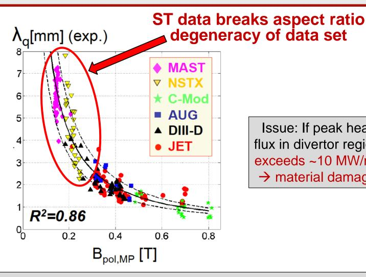
Issue: If peak heat flux in divertor region exceeds ~10 MW/m<sup>2</sup> → material damage
