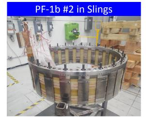
One bay w/ a complete set of new welds, brackets, "biscuits" & toroidal blocks
