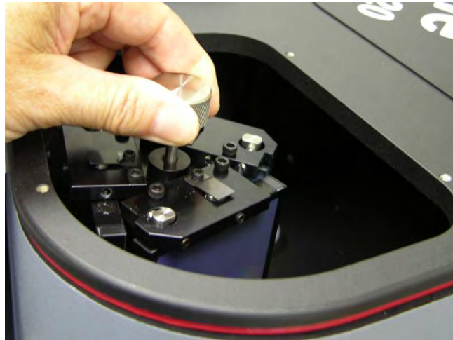
Figure 2-7. Lower Turret into the Turret Compartment
