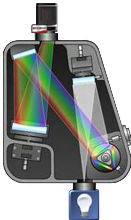
Figure 1-1. Light Path within the IsoPlane SCT 320
