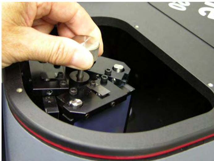
Figure 2-16. Lift Turret up out of the Turret Compartment
