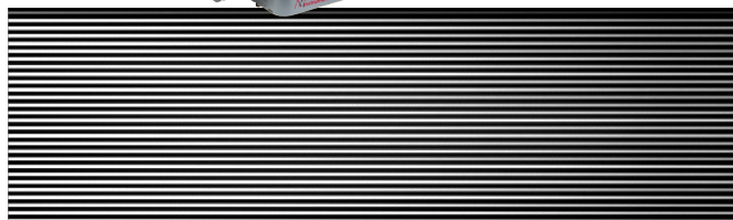
Images acquired with fourteen 100 \mu\text{m} fibers, white light source, 1340 x 400 CCD, 1200 g/mm grating blazed at 500 nm, first order.
