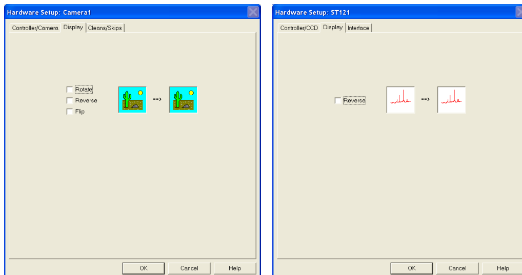
Figure 16. Display tab; left graphic applies to all controllers except ST-121; right graphic applies to ST-121 only
