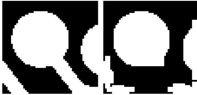
Figure 147. Original Image (left) and Opened Image with Three Iterations (right)
