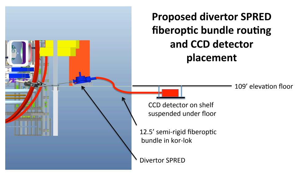
Motivation: need to remove CCD detector as far away from machine (magnetic field) as possible
