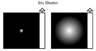
An Iris shutter opens in an expanding circular pattern.
