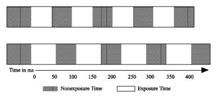
The first sequence runs with a filter that uses exposure and nonexposure times that are equal. In the second sequence, the exposure time is longer, but the time between exposures remains the same as in the first sequence.
