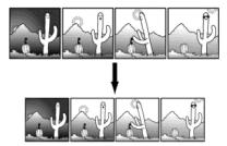
• Multiple Exposures, Multiple Images: A series of exposures with multiple regions. Each exposure must have identical regions. The data are stored in several image arrays that are stored inside a single buffer.
