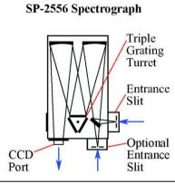
Figure 2. Includes a 90° optical path, large 14 mm X 27 mm focal plane, plus sliding tube CCD adapter with exclusive focus-stop.
