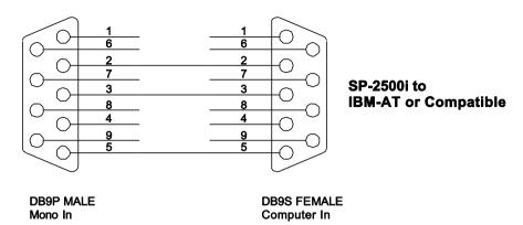
Figure 9. RS-232 Cable Wiring
