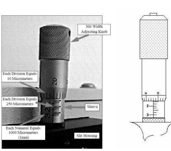
Figure 7. Slit Width Setting: 200 Micrometers (0.200 mm)
