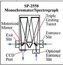
Figure 4. Includes dual exit ports; one exit slit and one sliding CCD adapter with motorized mirror for rapid, computer-controlled exit slit selection.
