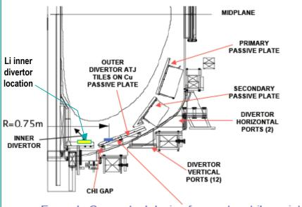
Example Conceptual design for a outer strike-point, horizontal toroidal annulus, Liquid Lithium Lower Divertor, ~10 cm wide x 2.5 cm deep, R<sub>m</sub>~0.75 m
