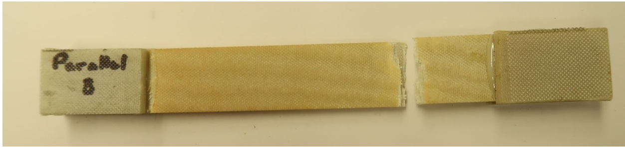
Figure 2.1.1-2: Photo of a failed dogbone sample
