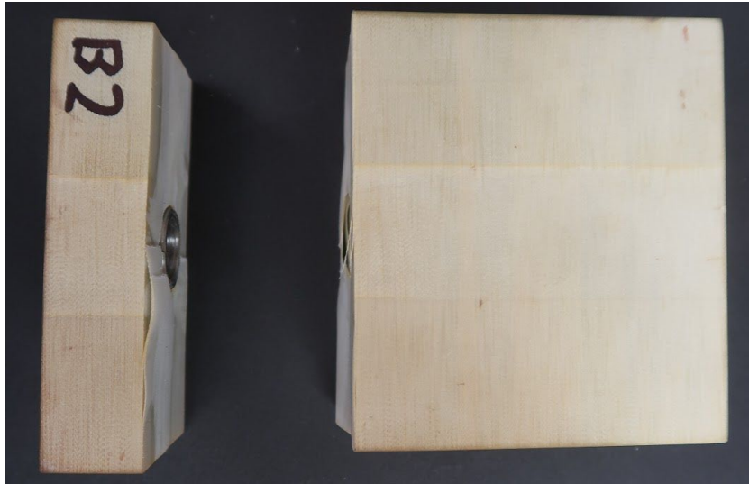
Figure 2.1.1-1: Photo of a failed double-keensert test.
