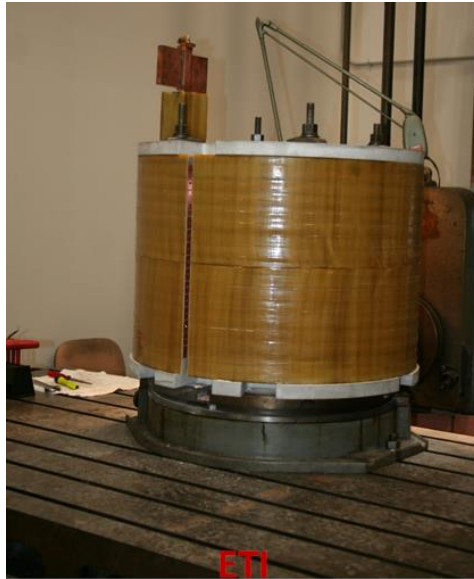
Figure 17: ETI and PPPL coils being sectioned on the Lucas milling machine
