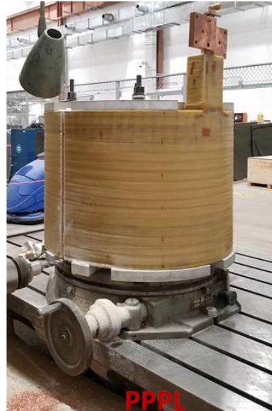
Figure 17: ETI and PPPL coils being sectioned on the Lucas milling machine
