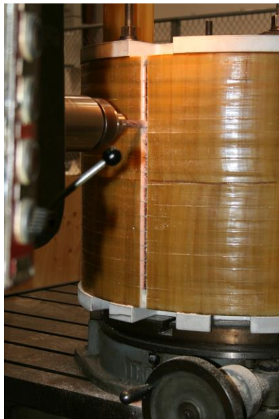
Figure 18: ETI (left) and PPPL coil (right) being sectioned on Lucas milling machine
