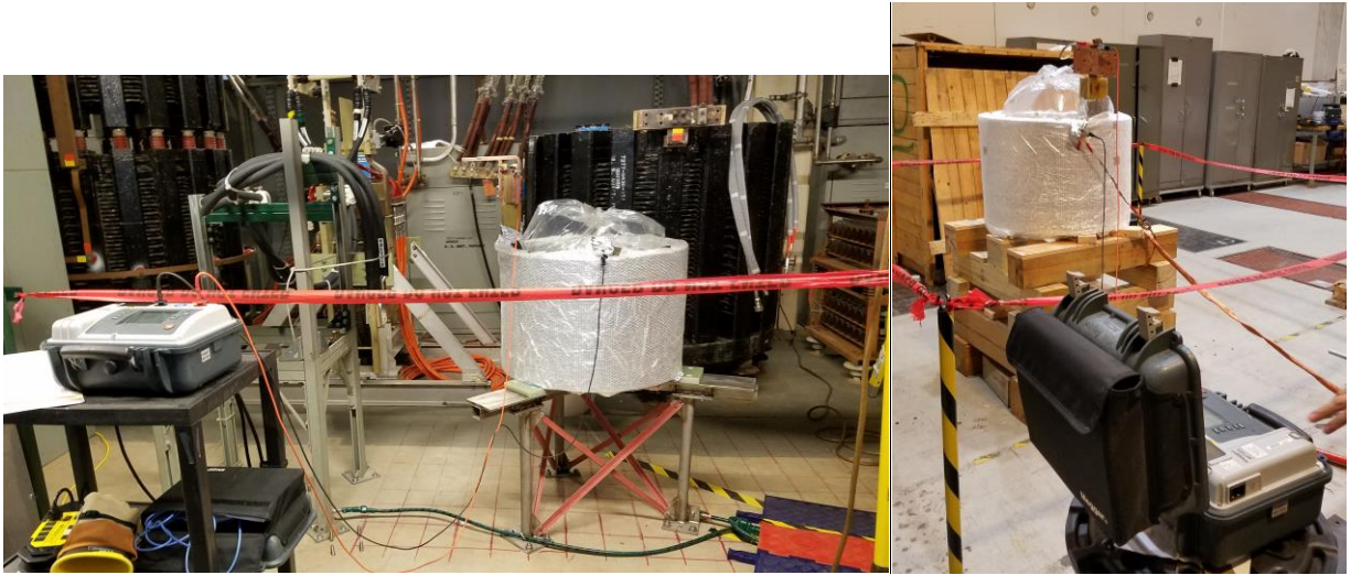
Figure 7: ETI (left at FCPC) coil and PPPL coil (right at coil shop) being high-pot tested relative to an applied ground plane
