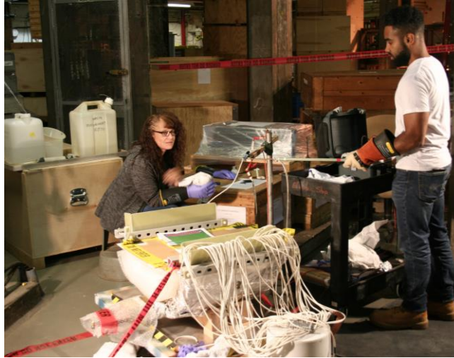
Figure 27: Turn-to-turn insulation resistance and hi-pot test of sectioned ETI PF-1aP coil
