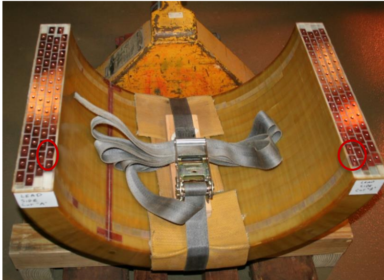
Figure 19: Sectioned ETI coil – No-lead section
