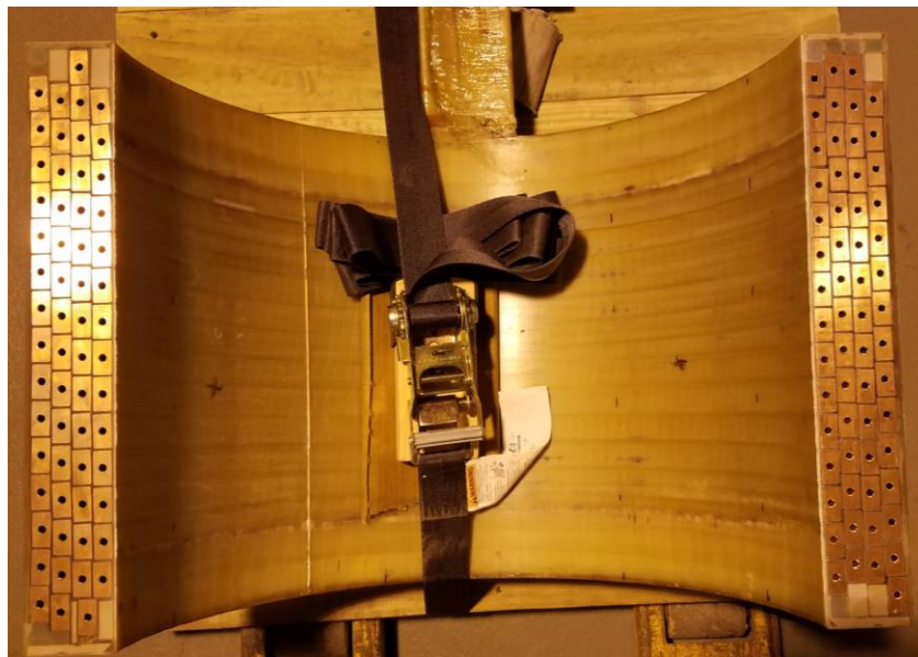
Figure 20: Sectioned PPPL coil – Lead section
