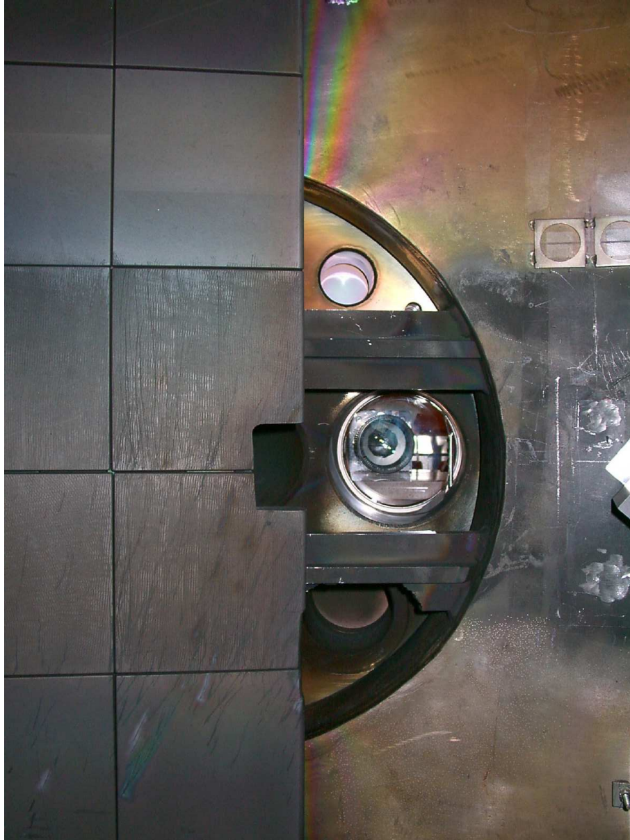
Fig. 15. In-vessel view of the MID CCD camera mounted at Bay I port 6" window. Neutral beam armor is on the left.
