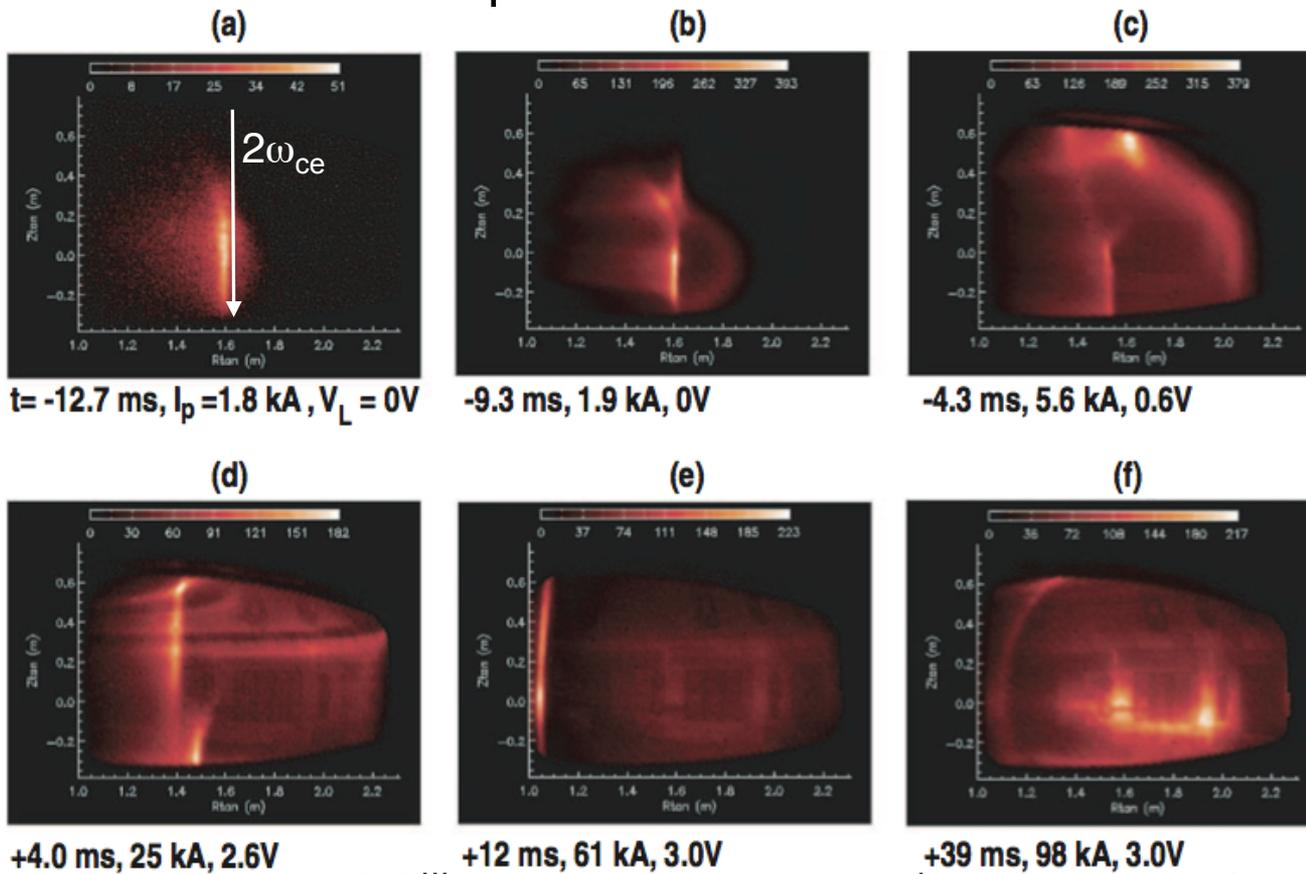
Fast-framing camera of C<sup>III</sup> emission during 2<sup>nd</sup> harmonic ECH in DIII-D
