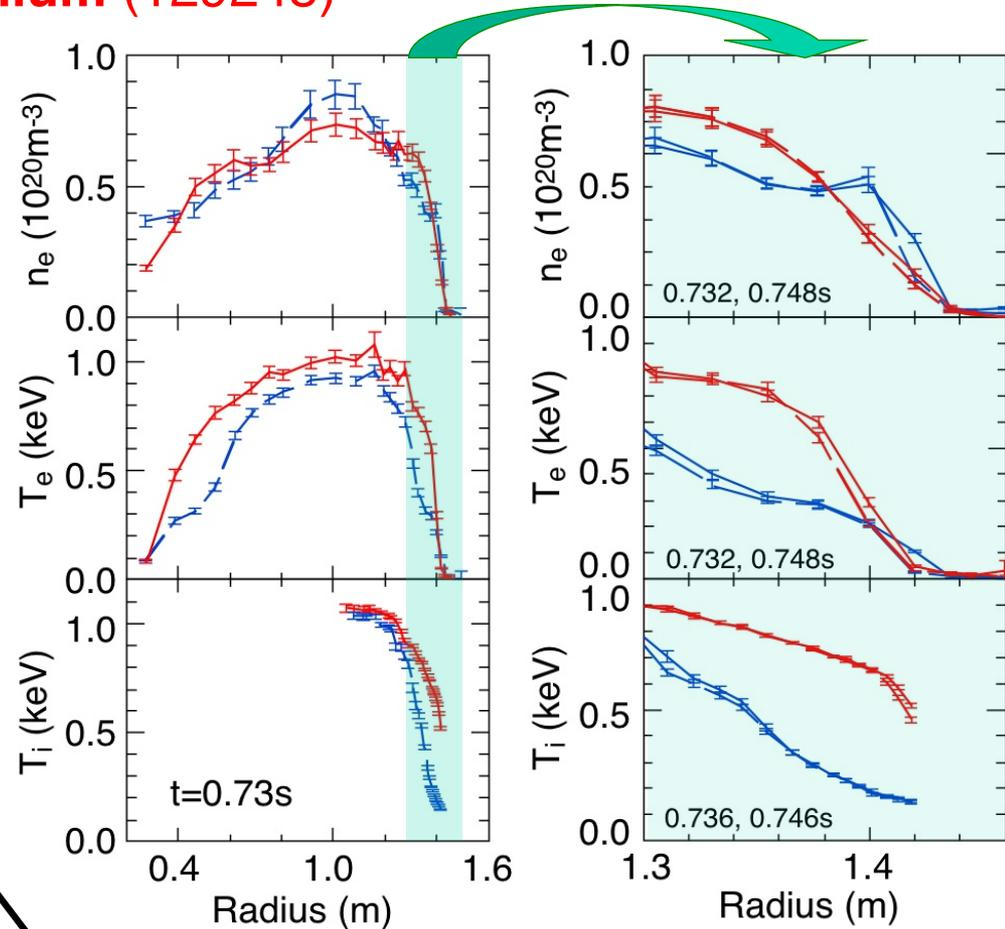
Without ELMs, impurity accumulation increases radiated power and  $Z_{eff}$
