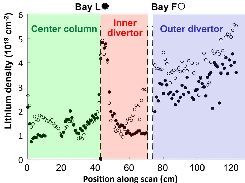
Peak lithium density remaining on inner divertor  $\sim 0.6 \text{ mg} \cdot \text{cm}^{-2}$
