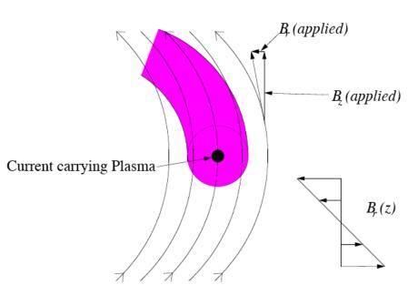
For a vertically stable plasma, as the plasma moves up, it encounters a radial field that pushes it down
