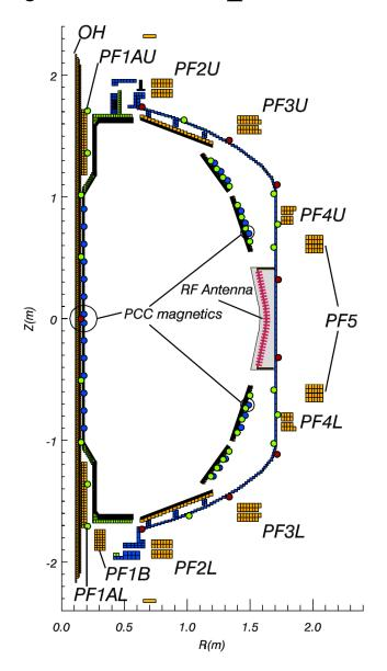
Picture showing the location of magnetic field coils and measurements used in real time reconstruction
