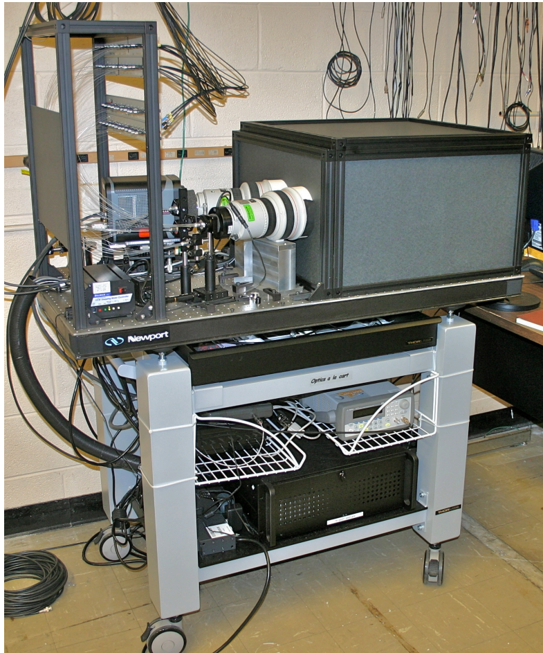
Spectrometer on mobile platform with computer and all associated hardware at LTX
