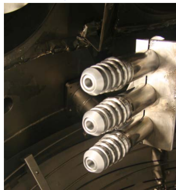
“Pagoda-style” injectors sustain V_{inj} \leq 1.5 \text{ kV} , I_{inj} \sim 2 \text{ kA} with no PMI effects within 1-2 cm of LCFS
