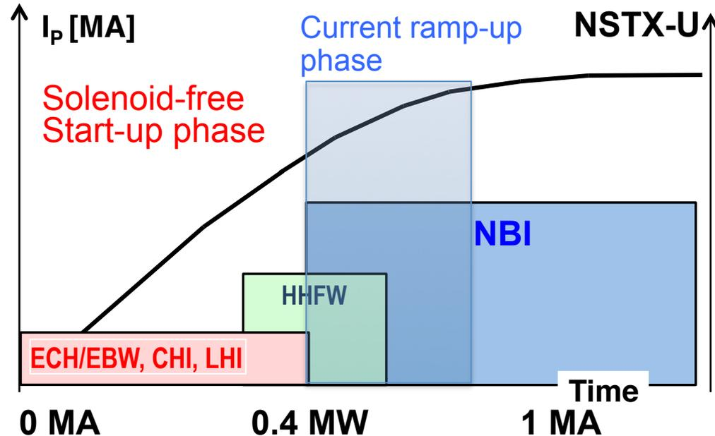
ECH / EBW – Utilize 1 – 2 MW 28 GHz gyrotron
