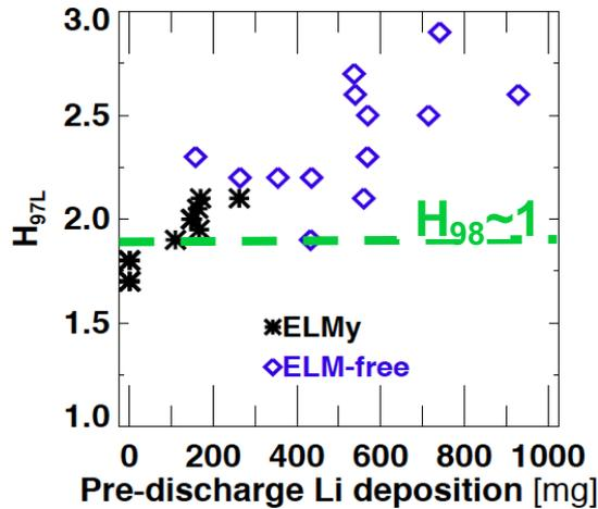
NSTX-U near-term: Double Li deposition, effect on confinement (carbon tiles)
