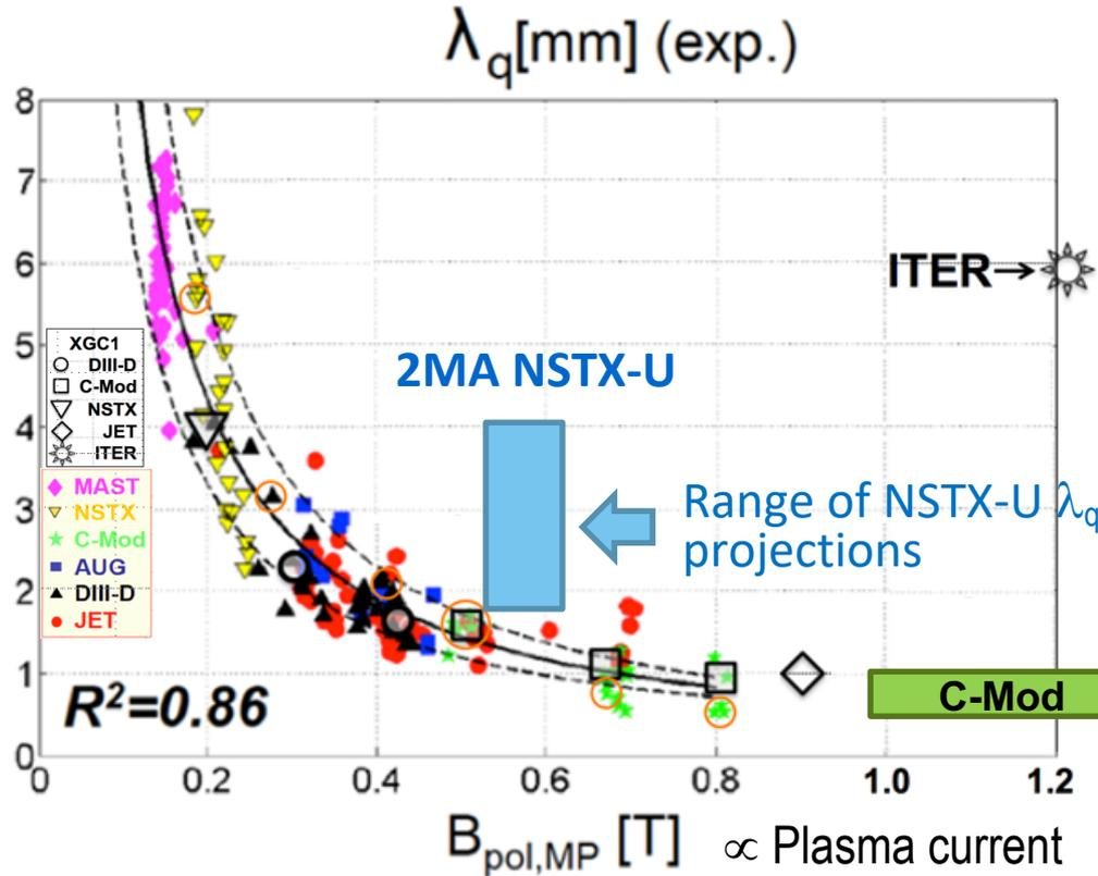
XGC1 simulations predict turbulence will widen edge heat flux in ITER
