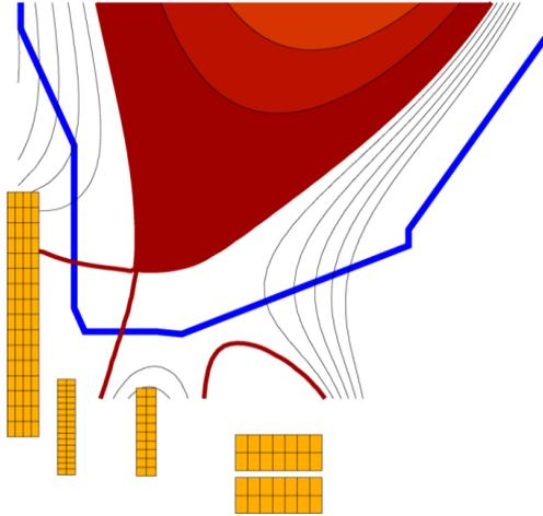
**New PF1 magnets for flaring control, highest shaping, highest ST edge parallel heat flux**
