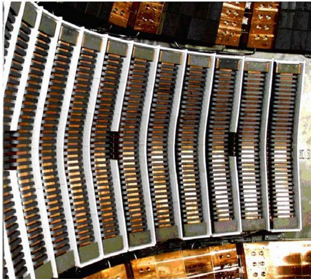
Figure 3.3.1 The twelve-strap HHFW antenna array.
