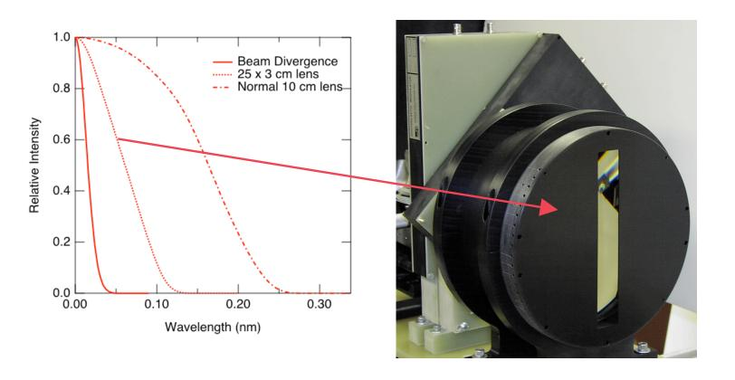
ullet Novel optics design, combined with high throughput, high resolution birefringent filter, can increase the polarization fraction to  $\sim 30\%$ .
